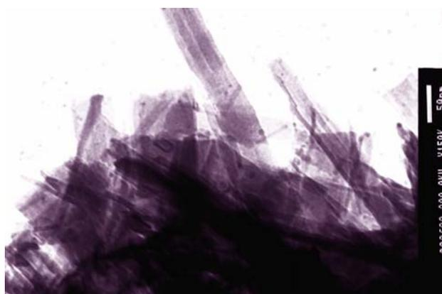
**Figure 1: TEM image of the light yellow-green precipitate (boltwoodite) collected from the experiment 1.1**
