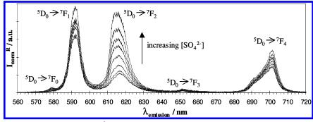
Figure 4. TRLIL spectra of Eu(III) with  $-4.1 < \log[SO_4^{2-}] < -1.6$ , in Na<sub>2</sub>SO<sub>4</sub>/NaClO<sub>4</sub> aqueous solutions with I = 0.5 M at  $-\log[H^+] > 3$  and 23 °C.
