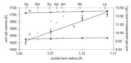
**Fig. 6.** Relationships between the ionic radii of the lanthanides [45] and the unit cell parameters of the corresponding Na $Ln(CO_3)_2$ ,  $xH_2O$  compounds. Our experimental data (solid black triangles) are compared with those of Mochizuki et al. (open grey lozenges) [31] and Runde et al. (solid grey lozenges) [37]. The determined relationships are:  $a = (11.10 + 1.75r_{Ln^{3+}})$ ,  $c = (8.60 + 1.13r_{Ln^{3+}})$  and  $V = (968 + 638r_{Ln^{3+}})$ .
