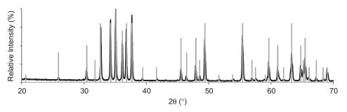
Fig. 2. XRD analysis of NaEu( $CO_3$ )<sub>2</sub>, 5H<sub>2</sub>O residuum after its thermal decomposition. The experimental pattern is in black, and JCPDS 00-012-0384 Eu<sub>2</sub>O<sub>3</sub> reference file is in grey.
