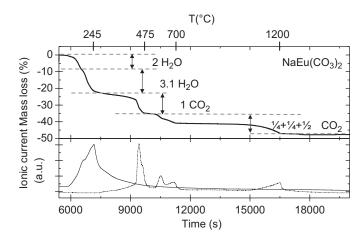
**Fig. 1.** Thermogravimetric and corresponding mass spectrometry analysis of NaEu(CO<sub>3</sub>)<sub>2</sub>, 5H<sub>2</sub>O. The weight loss is represented in the upper part of the graph and the emissions of water (solid line) and carbon dioxide (dashed line) are represented in the bottom part.
