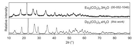
Fig. 5. Comparison of Dy<sub>2</sub>(CO<sub>3</sub>)<sub>3</sub>, xH<sub>2</sub>O diffraction pattern with Eu<sub>2</sub>(CO<sub>3</sub>)<sub>3</sub>, 3H<sub>2</sub>O referenced one.
