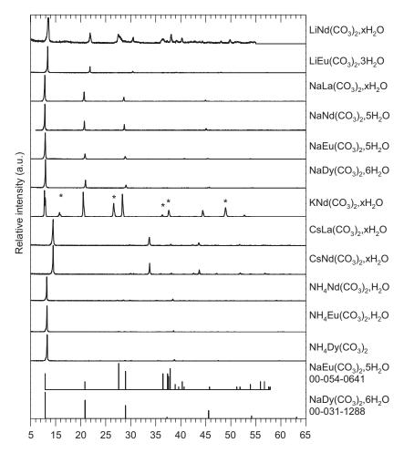
**Fig. 4.** Powder XRD patterns of hydrated  $ALn(CO_3)_2$ ,  $xH_2O$  solid compounds.
