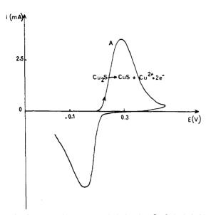
**Figure 1.** Current-voltage curve of chalcocite (Cu<sub>2</sub>S) included in a carbon paste electrode: Cu<sub>2</sub>S (0.3 mg); H<sub>2</sub>SO<sub>4</sub> 1 M (40 mg); carbon (50 mg); scan rate:  $10^{-3}$  V·s<sup>-1</sup>
