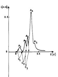
**Figure 2.** Current-voltage curve of chalcocite (Cu<sub>2</sub>S) included in a carbon paste electrode: Cu<sub>2</sub>S (0.6 mg); H<sub>2</sub>SO<sub>4</sub> 1 M (40 mg); carbon (50 mg); scan rate:  $10^{-4}$  V-s<sup>-1</sup>
