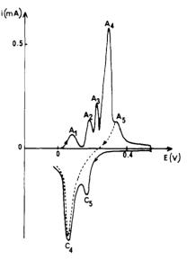
**Figure 3.** Current-voltage curve of chalcocite (Cu<sub>2</sub>S) included in a carbon paste electrode: Cu<sub>2</sub>S (0.6 mg);  $H_2SO_4$  1 M (40 mg); carbon (50 mg); scan rate:  $10^{-4}$  V·s<sup>-1</sup>
